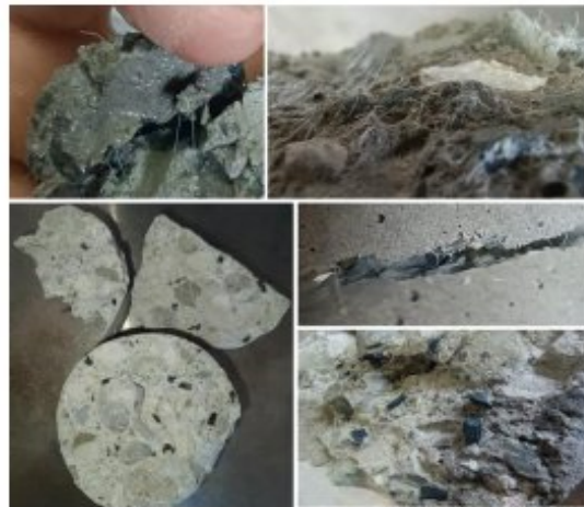
Figure 1. Distribution of PET fibers in concrete specimens, showing their integration and the overall homogeneity of the mixture. The image also highlights differences in compressive fracture behavior between specimens without PET fibers and those with fiber reinforcement, where the fibers help bridge aggregates and maintain structural integrity after failure.
